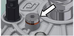
As soon as water comes from the vent without air, plug again the hole and top up the radiator.
