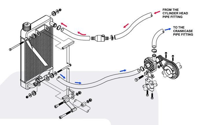
Filling the circuit (with pure water), be sure to provide proper air purging from the water pump and pipes. To purge the water jackets of cylinder and cylinder head remove the plug on the top of cylinder head while filling the radiator.
