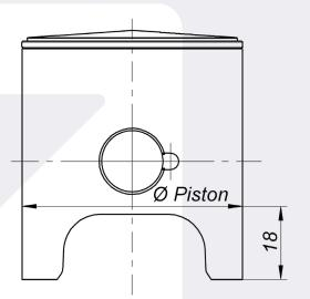
When it's not possible to verify the real piston diameter, the marking on piston top can be used to set the cylinder bore. If the marking on piston top is with the size plus:
